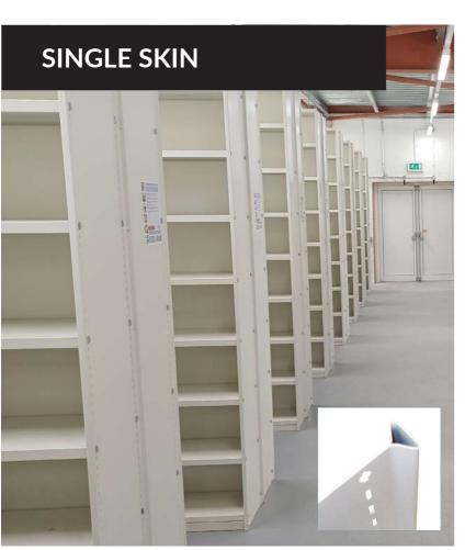
The Rackline Profile single-skin shelving system consists of a panel with a double-form rear section.
